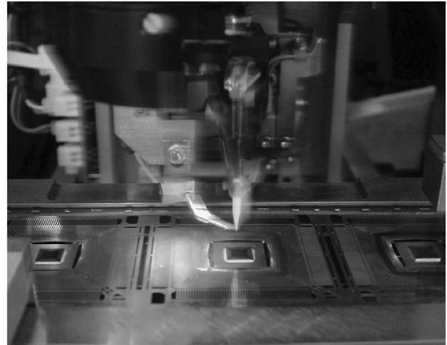
Fig. 3. Front view of the head of wire bonder.
